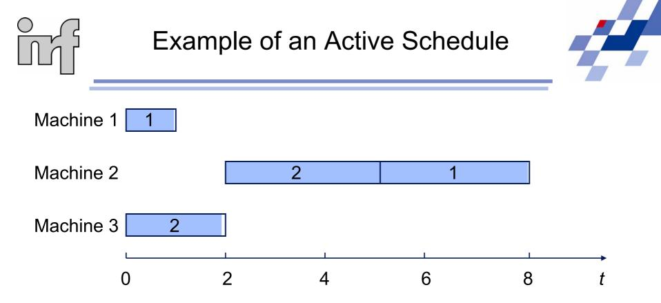
It is clear that this schedule is active as reversing the sequence of the two jobs on machine 2 postpones the processing of job 2. However, the schedule is neither nondelay nor optimal. Machine 2 remains idle until time 2 while there is a job available for processing at time 1.
