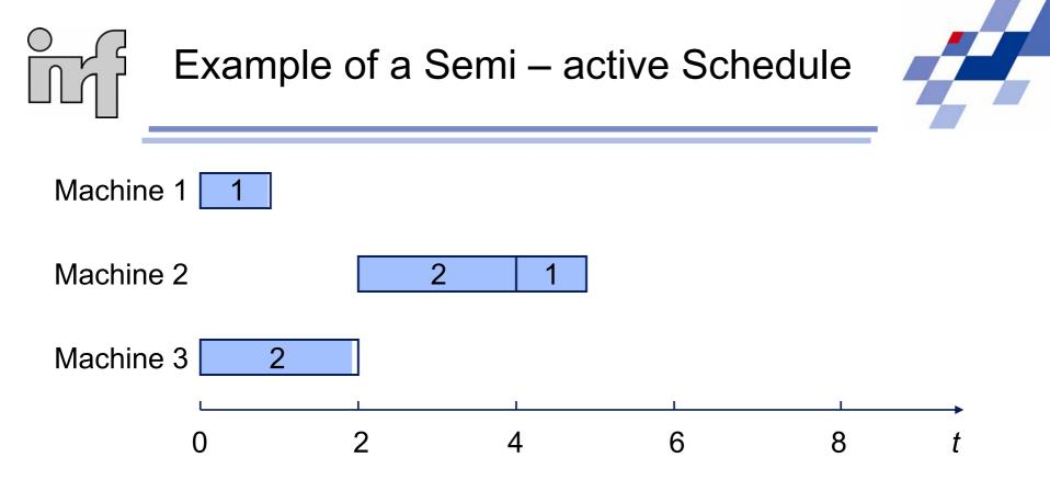
Consider the schedule under which job 2 is processed on machine 2 before job 1. This implies that job 2 starts its processing on machine 2 at time 2 and job 1 starts its processing on machine 2 at time 4. This schedule is semi-active. However, it is not active as job 1 can be processed on machine 2 without delaying the processing of job 2 on machine 2.
